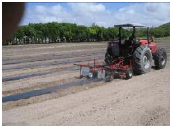
Plate 13: Laying drip lines and plastic mulch for West Indies Red hot pepper plot at Central Cotton Station, Antigua
