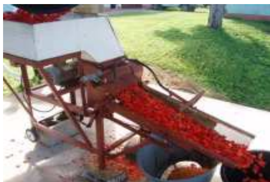
Plate 4 Mechanical seed extraction process
