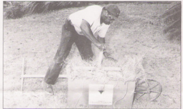
Fig. 4. Pressing Frame placed on top, handle placed into cradle of pressing frame...
