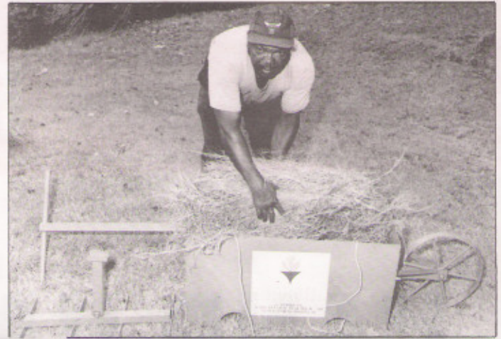
Fig. 3. Keep loading hay until about 12 - 15 cm (5 - 6 in) above chamber edge.
