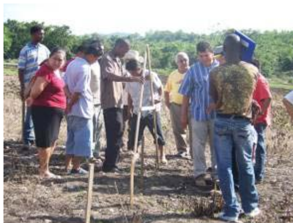
Plate 11: Participants (farmers) getting hands-on experience in marking contours using the "A" Frame
